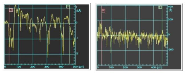
Figure 6: Surface profile scans of silicon wafer sample after polishing with 6 µm diamond suspension on ChemoTex<sup>™</sup> (left) and SanyPol<sup>™</sup> (right). The Ra was given as 463Å for sample 10 at left and 40Å for sample 9 at right.
