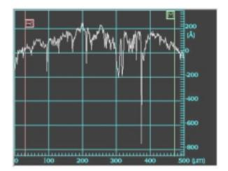
**Figure 7:** Surface profile scans of silicon wafer sample after polishing with 1 μm diamond suspension on Nylon (left) and Rayon Fine (right). The Ra was given as 24Å for sample 16 at left and 57Å for sample 6 at right.
