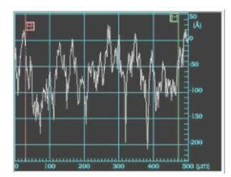
**Figure 8:** Surface profile scans of silicon wafer sample after polishing with 1 µm aluminum oxide suspension on MultiTex<sup>™</sup> (left) and Rayon Fine (right). The Ra was given as 94Å for sample 4 at left and 32Å for sample 5 at right.
