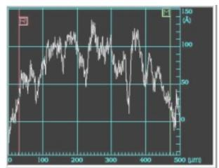
**Figure 9:** Surface profile scan of silicon wafer sample after polishing with 0.05 µm colloidal silica suspension on MultiTex<sup>™</sup>. The Ra was given as 22Å for sample 3.
