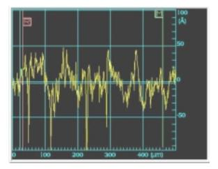
**Figure 2:** Surface profile scans of silicon wafer sample after polishing with 0.5μm (left) and 1 μm (right) diamond lapping films. The Ra was given as 15 and 17 Å, respectively.
