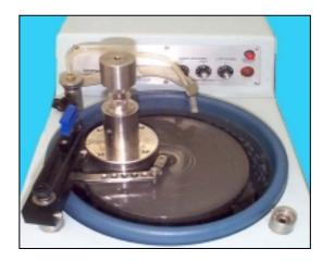
**Figure 1:** Image showing the basic arrangement used for polishing samples. The Model 920 Lapping and Polishing Machine is used with lapping plates, abrasive papers, abrasive films, or polishing cloths for sample preparation. The Model 155 Lapping and Polishing Fixture is pictured as well, which is used for holding samples and controlling thickness during processing.
