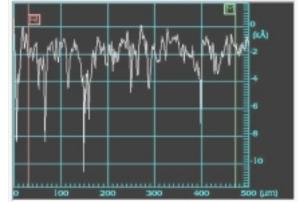
**Figure 4:** Surface profile scans of silicon wafer sample after lapping with diamond suspension on Cu composite plate using two different 15 µm diamond suspensions. The Ra was given as 608Å for sample 11 at left and 879Å for sample 13 at right.
