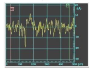
Figure 3: Surface profile scans of silicon wafer sample after lapping with aluminum oxide suspension on glass plate (left) and cast Fe plate (right). The Ra was given as 3140 and 3382 Å, respectively.
